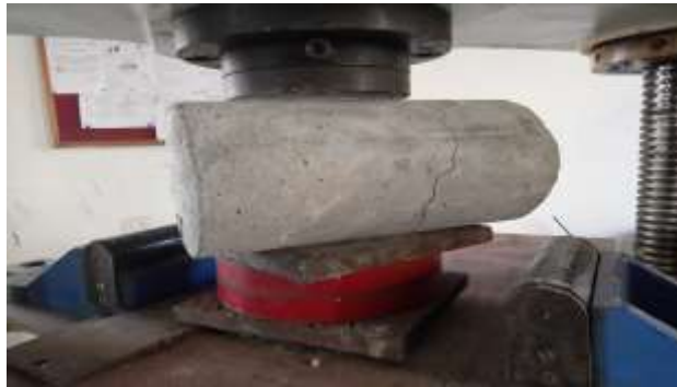
Figure 4.3.1: Splitting Tensile strength test setup
