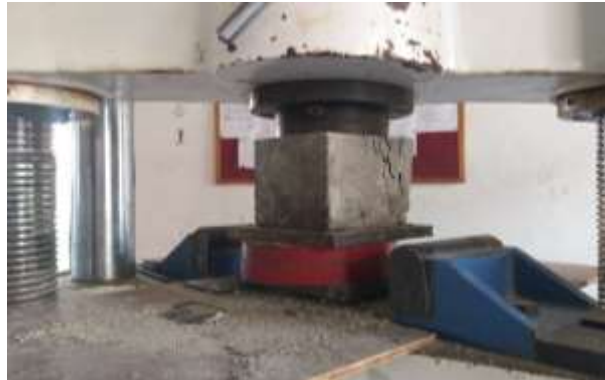
Figure 4.2.1: Compressive Strength test setup
