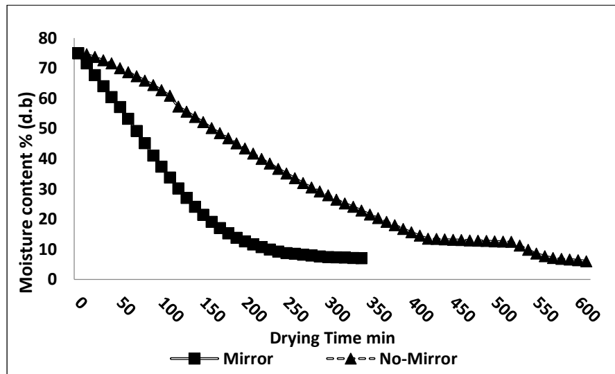
Fig(7) Variation in moisture content with mirror and without mirror
