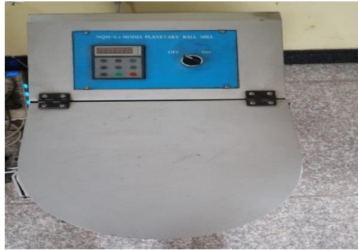
Figure1. Grind device used for milling teeth NQM-0.4 model planetary ball. (Yangzhou Nouya, China)
